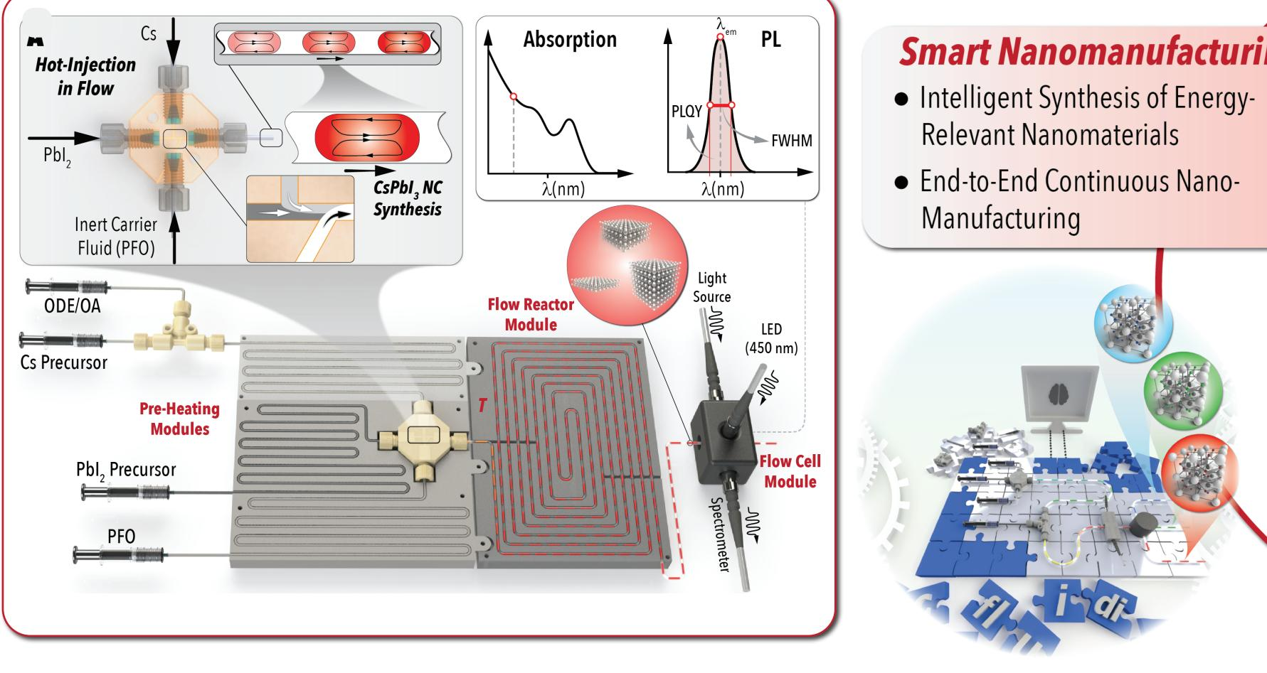
**Closed-Loop Autonomous Experimentation**
